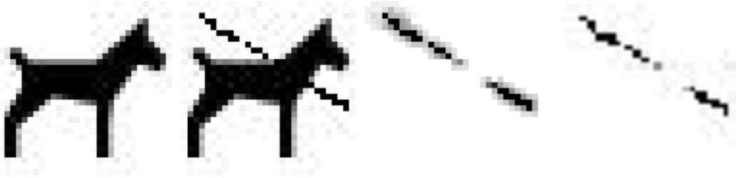
Fig. 4. An image and a modified version where a line has been introduced. The third image illustrates the dissimilarity (darkest gray levels). The global similarity is 0.96. The last image shows the inverted difference between the images (computed pixel-wise).
