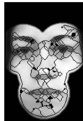
Fig. 3. Over-segmented image by the watershed algorithm.
