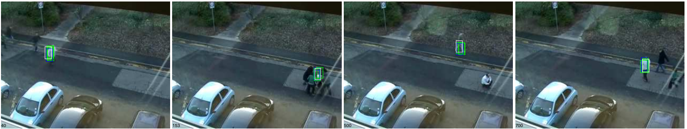
Fig. 7. seq. #1 Sample tracking results based on both color and motion with fixed reliabilities. The results are better than those that are obtained by considering single visual cues. However, this time a person entering the scene during which the actual person of interest is at rest results in inaccurate tracking.
