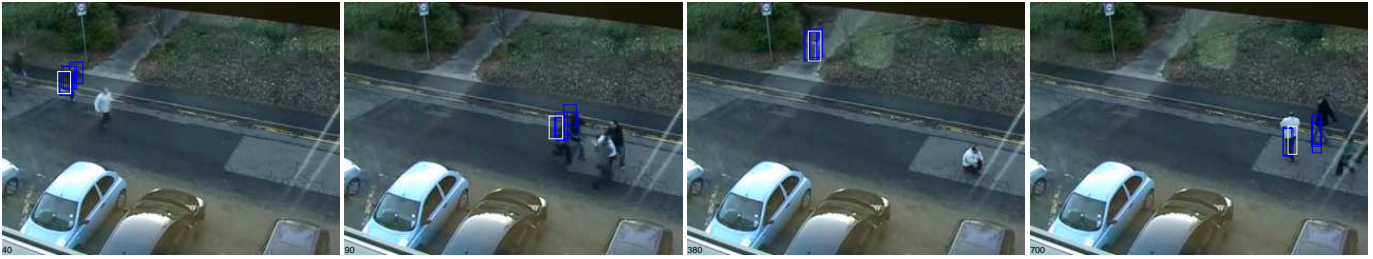
Fig. 6. seq. #1 Sample tracking results based on motion. The sequence contains several objects in motion, and thus during the tracking process the particles are distributed all around these objects instead of the actual object of interest.
