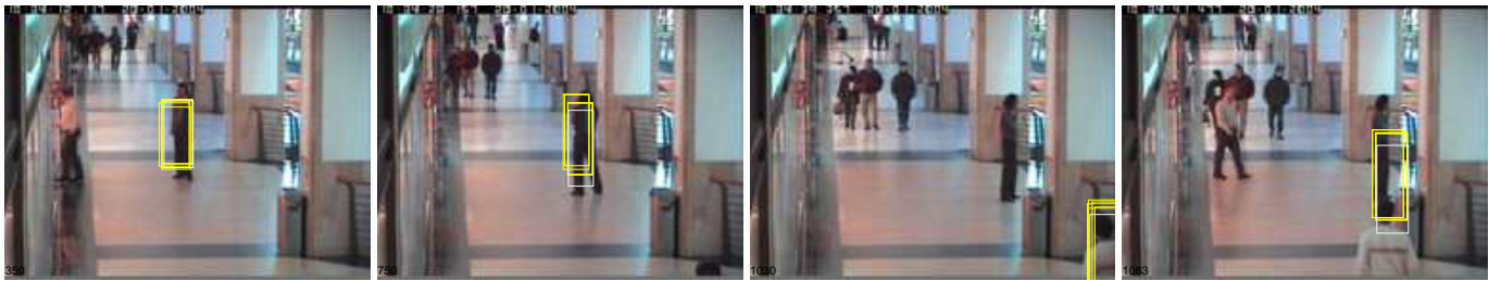
Fig. 18. seq. #3 Sample tracking results based on the two-layered partitioned sampling approach suggested by Perez et al. [18]. The video sequence involves several persons in motion, and since the localization of the person of interest is depend on primarily motion and then color information, the particles are distributed all around these persons.
