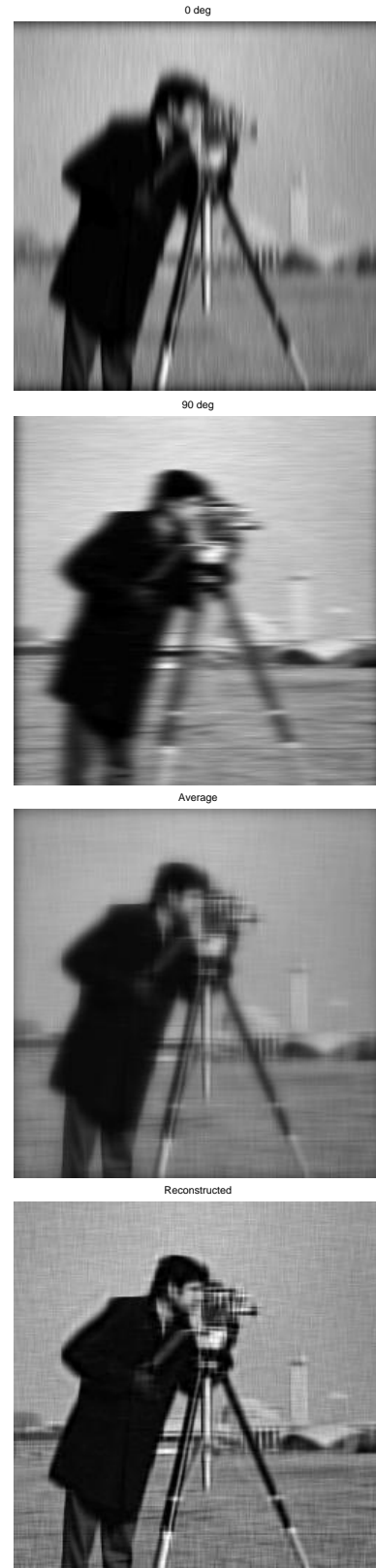
Figure 4. Image with synthetic degradation. From top to bottom: 1. Acquisition at 0 degree, 2. Acquisition at 90 degrees, 3. Average, 4. Reconstructed volume
